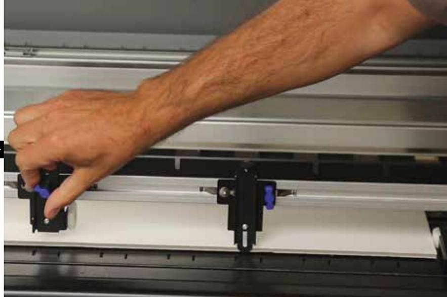
The ValueJet 1626UH in Mutoh's showroom is equipped with a new front loading system ensuring that plate material can be positioned even more accurately.
